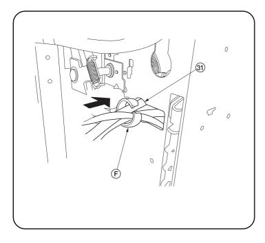
14. Pass the cable to be passed through the connection hole (3) at the rear right of the main body through the Open Bushing, OCB-1000 (F), and fit it to the connection hole (3).
