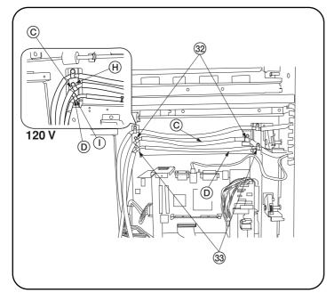
**15A. (120 V specifications)** Set the shaded area <sup>(2)</sup> of the Junction Wiring A, Interface PCB <sup>(C)</sup> with the clamp, GNK-5N <sup>(H)</sup> and the shaded area <sup>(3)</sup> of the Junction Wiring B, Interface PCB <sup>(D)</sup> with the clamp, EMT-3N <sup>(I)</sup>, and fix them with four binding screws M4 x 6 <sup>(J)</sup>.
