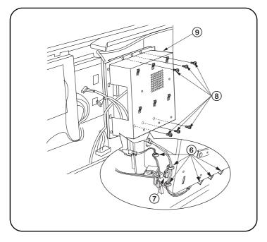
**19.** Fit the controller cover with six screws (a), lock the lower left six clamps (b) on the right controller cover from the rear side of the main body, and connect the connector (7).
