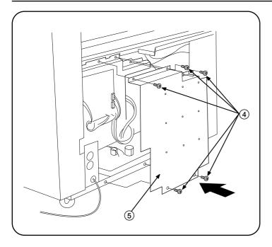
**18.** Reattach the main-PCB cover (5) with 5 screws (4).
