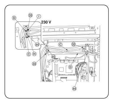
**15B. (230 V specifications)** Bind the Shaded area of the Junction Wiring A, interface PCB ⓒ with the CLAMP, GNK-5N ⊕ and at the upper right ② and at the lower left ③, fix it with two binding screws M4x6 ④.
