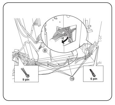
9. Put the 9-pin connector side of the Junction Wiring and Printer Unit (B) near the main PCB and the 6-pin connector side near the right side of the controller unit, and then lock the wire saddle (9) at seven locations and lay it down.
