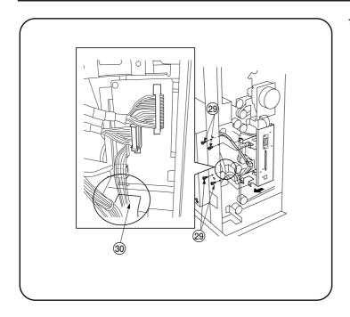
12. Connect the modular connector @, Junction Wiring, Printer Unit (B)10-pin connector @, 6-pin connector @ (on the front side of Scanner Interface PCB Assembly), Junction Wiring B, Interface PCB (D)?, and Junction Wiring A, Interface PCB (C)? to the Scanner Interface PCB Assembly (E) described in step 11.
