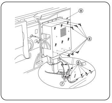
**3.** From the rear side of the main body, unlock the clamp (6) at the lower left of the controller cover located at the right side, remove the connector (7) and the six screws (8), and then remove the controller cover (9).
